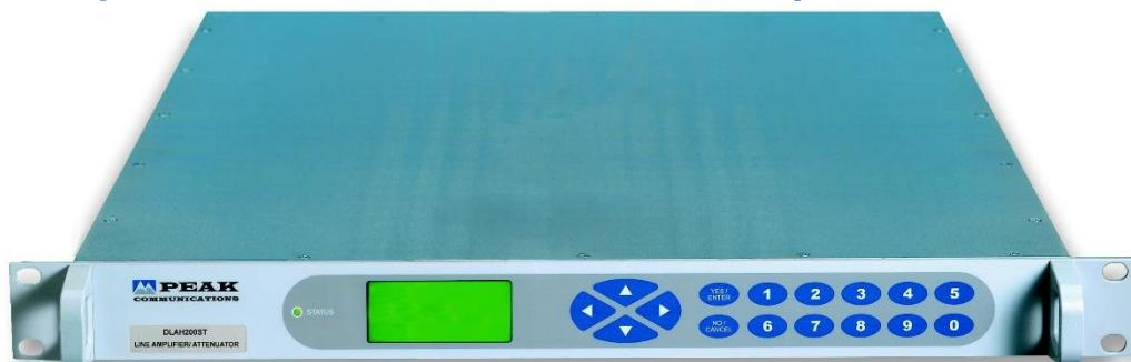
The 19-inch 1U rack mounted **DBUH200(Ka)** chassis unit is designed to accept any mix of two of the converter modules shown below. Modules can be inserted/ replaced in the **DBUH200(Ka)** unit from the rear without the need to remove power or disturb the other channel in any way.
