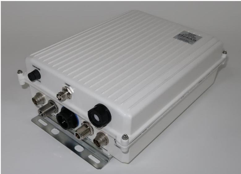
The **PBU(Ka) series** remote mounted, block up converter units from Peak Communications are designed to be fully compatible with a wide range of L-Band modulators and frequency converters. This high-grade range of **PBU** outdoor units will accept the L-band output of a **P7000 series** up converter or modem and provide the frequency conversion to Ka bands.
