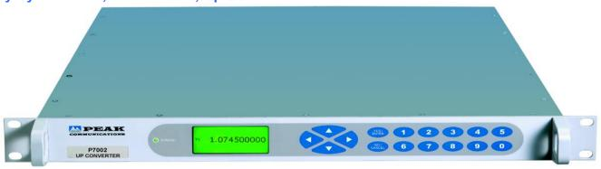
The P7002 is a next generation fully synthesised L-Band up converter which provides a low-cost solution for systems requiring an IF interface at 70MHz ±18MHz, 140MHz ±36MHz or switchable between 70 & 140MHz.
