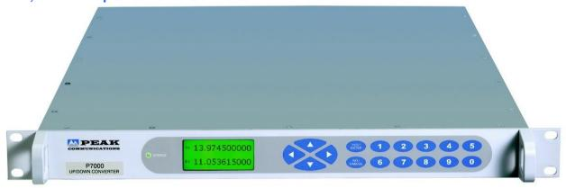
The P7020 is a next generation fully synthesised combined S-Band up and down converter which provides a low-cost solution for systems requiring an IF interface at 70MHz ±18MHz or 140MHz ±36MHz. The unit incorporates a graphics display module, membrane keyboard and features a clear and intuitive control and configuration menu fully utilising the unique graphics display.
