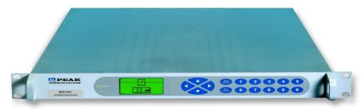
The 19-inch 1U rack mounted IBDH(A) series of block frequency down converter units from Peak Communications are designed to take the incoming SHF signal and produce an output at L-Band that is suitable for direct connection to an L-band demodulator or for further conversion typically by a P7001 synthesised down converter.
