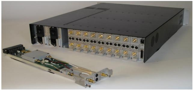
The VGU010 system provides fixed gain &/ or attenuation control of IF, L-Band & SHF based signals, which can be used for balancing during commissioning to overcome differences in cross-site cable losses, as well as providing a useful facility for earth station operators to adjust the gain of uplink/ downlink chains remotely. SHF units can be used for coverage and capacity layer testing for 5G networks.
