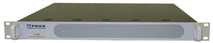
The **F1200** is a fixed frequency, fixed gain, combined L-Band Up and Downconverter. The **F1200** provides a low-cost solution for systems requiring conversion between 70MHz  $\pm$ 20MHz (or 140MHz  $\pm$ 40MHz) and L-Band. The unit can be used to interface L-Band modems with 70/140MHz transceivers or 70/140MHz modems to L-band transceivers.
