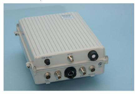
The F1201R is a remote mounted version of the popular Peak F1201 fixed frequency, fixed gain L-Band DownConverter which provides a low-cost solution for systems requiring conversion between L-Band and  $70 \text{MHz} \pm 20 \text{MHz}$  (or  $140 \text{MHz} \pm 40 \text{MHz}$ ). The unit is popular for interfacing L-Band modems with 70/140 MHz transceivers or 70/140 MHz modems to L-band transceivers.
