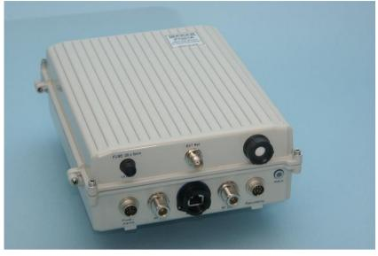
The P7001R is a remote mounted version of the popular Peak P7001 fully synthesised L-Band down converter which provides a low-cost solution for systems requiring an IF interface at 70MHz ±18MHz or 140MHz ±36MHz.
