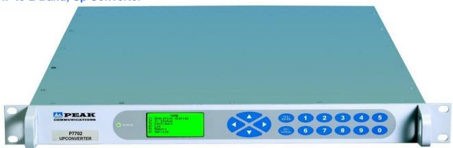
The 19-inch, 1RU rack mounted P7702i block up converter unit from Peak Communications is designed to typically take the incoming UHF signal and produce an output at L-Band that is suitable for further conversion by a P7001 converter or for direct connection to a receiver in a down link chain.
