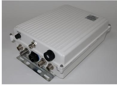
The remote mounted **PBD(B)** series of multi-range block frequency down converter units are designed to take the incoming SHF signal and produce an output at L-Band that is suitable for direct connection to an L-band demodulator or for further conversion typically by a **P7001** synthesised down converter.
