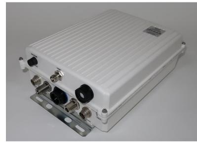
The **PBD(Ka)** series remote mounted, block down converter units from Peak Communications are designed to be fully compatible with a wide range of L-Band modulators and frequency converters. The high-grade range of **PBD(Ka)** outdoor units will accept the SHF input from an LNA system and provide a frequency conversion to L-Band.
