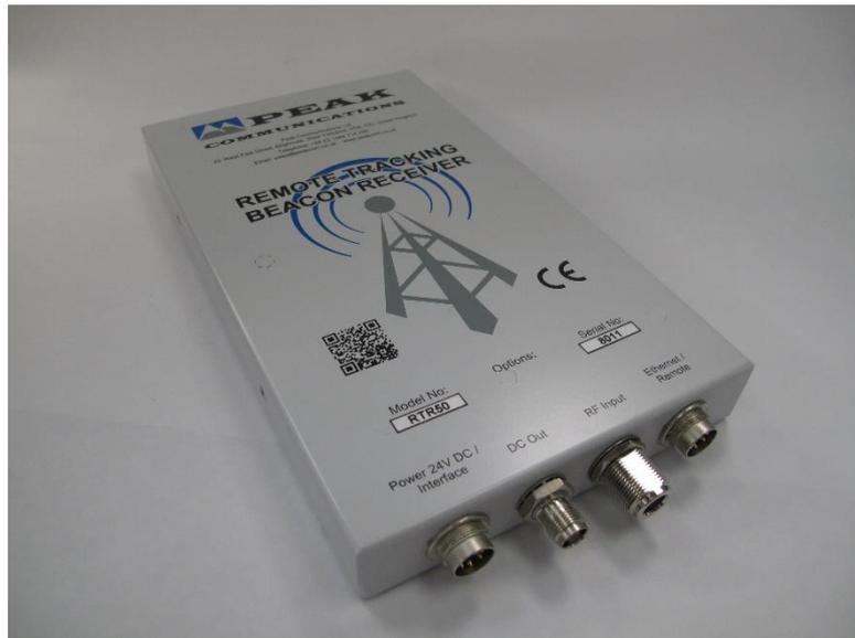
The **RTR51** is a next generation remote mounted tracking receiver, designed specifically to track and measure 'CW' beacons from commercial satellites. Primarily an L-Band input receiver, the unit is designed to be used for telemetry and control, typically in earth stations using medium to large antennae or for smaller antenna in typically SOTM /mobile applications.
